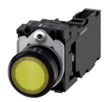
Illuminated pushbutton, 22 mm, round, plastic, yellow, pushbutton, flat, momentary contact type, with holder, 1 NO+1 NC, LED module with integrated LED 24 V AC/DC, screw terminal, Z=20-unit packaging
