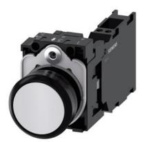
Pushbutton, 22 mm, round, plastic, white, pushbutton, flat, momentary contact type, with holder 1 NO+1 NC, spring-type terminal, with laser labeling, upper case
