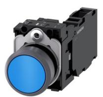
Pushbutton, 22 mm, round, plastic with metal front ring, blue, pushbutton, flat, momentary contact type, with holder, 1 NO+1 NC, screw terminal, with laser labeling, symbol number according to, ISO 7000 or IEC 60417
