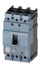
circuit breaker 3VA5 UL frame 125 breaking capacity class H 65kA @ 480 V 3-pole, line protection TM230, FTAM, In=40A overload protection Ir=40A fixed short-circuit protection Ii=5...10 x In UL489 SB (naval), 50 deg. cel. cable connection on both sides
