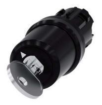
key-operated switch Siemens, 22 mm, round, plastic, lock number SSG10, with 2 keys, 2 switch positions O<I, momentary contact type, actuating angle 45°, 10:30h/12h, key removal O, with laser labeling, lower case
