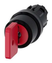
Key-operated switch O.M.R, 22 mm, round, plastic, lock number 73037, red, with 2 keys, 3 switch positions I>O<II, momentary contact type, actuating angle 2x45°, 10:30h/12h/13:30h, key removal O, with laser labeling, inscription or symbol Customer-specific selection with SIRIUS ACT configurator (CIN)
