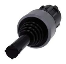
Coordinate switch, 22 mm, round, plastic with metal front ring, black, 2 switch positions, vertical latching, without mechanical interlocking, with laser labeling, upper case and lower case, always upper case at the beginning of the word
