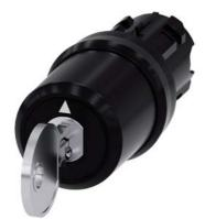
key-operated switch Siemens, 22 mm, round, plastic, lock number SSG10, with 2 keys, 3 switch positions I>O<II, momentary contact on the left, latching on the right, actuating angle 2x45°, 10:30h/12h/13:30h, key removal II, with laser labeling, upper case and lower case, always upper case at beginning of line
