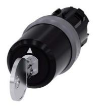
Key-operated switch BKS, 22 mm, round, plastic with metal front ring, special lock, with 2 keys, 3 switch positions I-O-II, latching, actuating angle 2x45°, 10:30h/12h/13:30h, key removal I, Note: BKS locking systems E1 - E25 supplied without key
