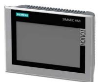
SIMATIC HMI TP700 Comfort INOX, Stainless steel front, Con- tinuous decorative film, Degree of protection front IP66K, 7" widescreen TFT display, PROFINET interface, MPI/PROFIBUS DP interface, 12 MB configuration memory, Windows CE 6.0, (Microsoft Support included Security updates discontinued) configurable from WinCC Comfort V11
