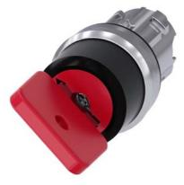
Key-operated switch O.M.R, 22 mm, round, metal, shiny, lock number 73037, red, with 2 keys, 2 switch positions O-I, latching, actuating angle 90°, 10:30h/13:30h, key removal O, with laser labeling, upper case and lower case, always upper case at beginning of line
