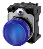
Indicator lights, 22 mm, round, metal, shiny, blue, lens, smooth, with holder, LED module with integrated LED 110 V AC, screw terminal, with laser labeling, inscription or symbol Customer-specific selection with SIRIUS ACT configurator (CIN)
