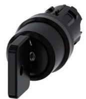
Key-operated switch O.M.R, 22 mm, round, plastic, lock number 73034, black, with 2 keys, 3 switch positions I>O<II, momentary contact type, actuating angle 2x45°, 10:30h/12h/13:30h, key removal O, with laser labeling, inscription or symbol Customer-specific selection with SIRIUS ACT configurator (CIN)
