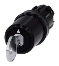
key-operated switch Siemens, 22 mm, round, plastic, lock number SSG10, with 2 keys, 3 switch positions I>O<II, momentary contact on the left, latching on the right, actuating angle 2x45°, 10:30h/12h/13:30h, key removal II, with laser labeling, inscription or symbol customer-specific selection with SIRIUS ACT configurator (CIN)
