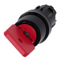
Key-operated switch O.M.R, 22 mm, round, plastic, lock number 73037, red, with 2 keys, 2 switch positions O-I, latching, actuating angle 90°, 10:30h/13:30h, key removal O, with laser labeling, upper case and lower case, always upper case at beginning of line
