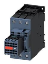
power contactor, AC-3 40 A, 18.5 kW / 400 V 2 NO + 2 NC, 24 V DC with varistor, 3-pole, Size S2, spring-type terminal, Captive auxiliary switch Suitable for 2 A PLC outputs
