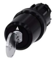
Key-operated switch BKS, 22 mm, round, plastic, lock number S1, with 2 keys, 3 switch positions I-O<II, left latching, right momentary contact type, actuating angle 2x45°, 10:30h/12h/13:30h, key removal O+I, with laser labeling, inscription or symbol Customer-specific selection with SIRIUS ACT configurator (CIN)
