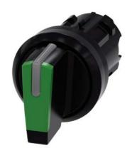
Selector switch, illuminable, 22 mm, round, plastic, green, selector switch, short, 3 switch positions I-O<II, left latching, right momentary contact type, actuating angle  $2x45^{\circ}$ , 10:30h/12h/13:30h, with laser labeling, upper case
