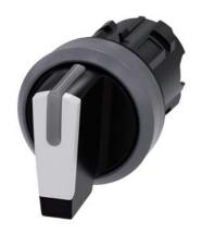
Selector switch, illuminable, 22 mm, round, plastic with metal front ring, white, selector switch, short, 3 switch positions I>O<II, momentary contact on the left, latching on the right, actuating angle 2x45°, 10:30h/12h/13:30h, with laser labeling, lower case
