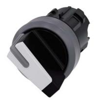
Selector switch, illuminable, 22 mm, round, plastic with metal front ring, white, selector switch, short, 2 switch positions O-I, latching, actuating angle 90°, 10:30h/13:30h, with laser labeling, upper case and lower case, always upper case at beginning of line
