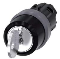
RONIS key-operated switch, 22 mm, round, plastic with metal front ring, special lock, with 2 keys, 3 switch positions I-O-II, latching, actuating angle 2x45°, 10:30h/12h/13:30h, Key removal II, possible special locks: SB31, 421, 455
