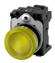
Indicator lights, 22 mm, round, metal, shiny, yellow, lens, smooth, with holder, LED module with integrated LED 230 V AC, spring-type terminal, Z=20-unit packaging
