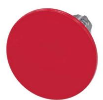
Mushroom pushbutton, 22 mm, round, metal, shiny, red, 60 mm, latching, pull-to-unlatch mechanism, with laser labeling, upper case and lower case, always upper case at beginning of line
