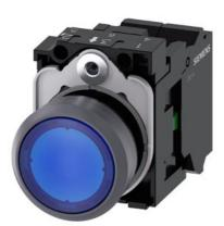
Illuminated pushbutton, 22 mm, round, plastic with metal front ring, blue, pushbutton, flat, momentary contact type, with holder, 1 NO, LED module with integrated LED 24 V AC/DC, Spring-type terminal
