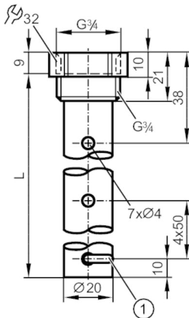
1 fixing bracket for centring piece
