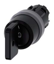
Key-operated switch O.M.R, 22 mm, round, plastic with metal front ring, lock number 73034, black, with 2 keys, 3 switch positions I-O-II, latching, actuating angle 2x45°, 10:30h/12h/13:30h, key removal O, with laser labeling, upper case and lower case, always upper case at beginning of line
