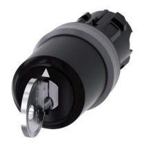
Key-operated switch IKON, 22 mm, round, plastic with metal front ring, lock number 360012K1, with 2 keys, 3 switch positions I-O<II, left latching, right momentary contact type, actuating angle 2x45°, 10:30h/12h/13:30h, key removal O+I, with laser labeling, upper case and lower case, always upper case at the beginning of the word
