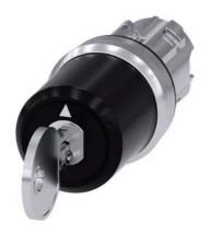
key-operated switch Siemens, 22 mm, round, metal, shiny, lock no. STGH10, with 2 keys, 3 switch positions I>O<II, momentary contact type, actuating angle 2x45°, 10:30h/12h/13:30h, key removal O, with laser labeling, upper case and lower case, always upper case at the beginning of the word
