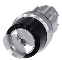
RONIS key-operated switch, 22 mm, round, metal, shiny, lock number 455, with 2 keys, 2 switch positions O-I, latching, actuating angle 90°, 10:30h/13:30h, key removal O+I, with laser labeling, upper case and lower case, always upper case at the beginning of the word
