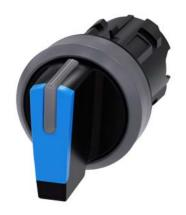
Selector switch, illuminable, 22 mm, round, plastic with metal front ring, blue, selector switch, short, 3 switch positions I>O<II, momentary contact on the left, latching on the right, actuating angle 2x45°, 10:30h/12h/13:30h, with laser labeling, upper case
