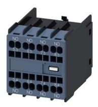
Auxiliary switch on the front, 4 NO Current path 1 NO, 1 NO, 1 NO, 1 NO for contactor relays Size S00 spring-type terminal 53/54, 63/64, 73/74, 83/84 Physically coded; only with contactor relays 3RH2140\* and 3RH2440\* can be combined (according to EN 50011)
