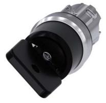
Key-operated switch O.M.R, 22 mm, round, metal, shiny, lock number 73034, black, with 2 keys, 2 switch positions O-I, latching, actuating angle  $90^{\circ}$ , 10:30h/13:30h, key removal O+I, with laser labeling, lower case
