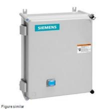
Non-reversing motor starter, Size 2, Three phase full voltage, Solid-state overload relay, OLR amp range 13-52A, Non-combination type, Enclosure type 4X fiberglass, Water/dust tight noncorrosive, Standard width enclosure
