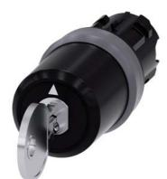
key-operated switch Siemens, 22 mm, round, plastic with metal front ring, lock number SSG10, with 2 keys, 3 switch positions I>O<II, momentary contact on the left, latching on the right, actuating angle 2x45°, 10:30h/12h/13:30h, key removal O+II, with laser labeling, upper case
