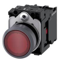
Illuminated pushbutton, 22 mm, round, plastic with metal front ring, red, pushbutton, flat, momentary contact type, with holder, 1NC, LED module with integrated LED 24 V AC/DC, screw terminal, with laser labeling, symbol number according to, ISO 7000 or IEC 60417
