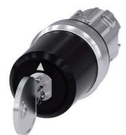
Key-operated switch BKS, 22 mm, round, metal, shiny, lock number S1, with 2 keys, 3 switch positions I>O<II, momentary contact on the left, latching on the right, actuating angle  $2x45^{\circ}$ , 10:30h/12h/13:30h, key removal O, with laser labeling, lower case
