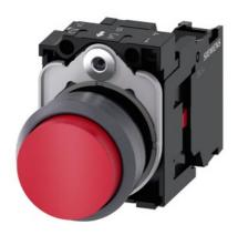
Pushbutton, 22 mm, round, plastic with metal front ring, red, pushbutton, raised, momentary contact type, with holder, 1 NC, screw terminal, Z=20-unit packaging
