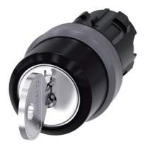
RONIS key-operated switch, 22 mm, round, plastic with metal front ring, lock number SB30, with 2 keys, 3 switch positions I-O-II, latching, actuating angle 2x45°, 10:30h/12h/13:30h, Key removal I+O+II, possible special locks: SB31, 421, 455, with laser labeling, inscription or symbol Customer-specific selection with SIRIUS ACT configurator (CIN)
