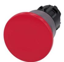
Mushroom pushbutton, 22 mm, round, plastic with metal front ring, red, 40mm, momentary contact type, with laser labeling, symbol number according to, ISO 7000 or IEC 60417
