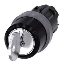
RONIS key-operated switch, 22 mm, round, plastic with metal front ring, special lock, with 2 keys, 3 switch positions I-O-II, latching, actuating angle 2x45°, 10:30h/12h/13:30h, Key removal I+O+II, possible special locks: SB31, 421, 455
