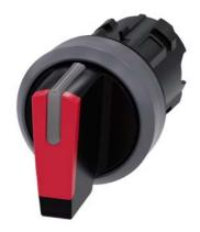
Selector switch, illuminable, 22 mm, round, plastic with metal front ring, red, selector switch, short, 3 switch positions I>O<II, momentary contact on the left, latching on the right, actuating angle 2x45°, 10:30h/12h/13:30h, Z=50-unit packaging
