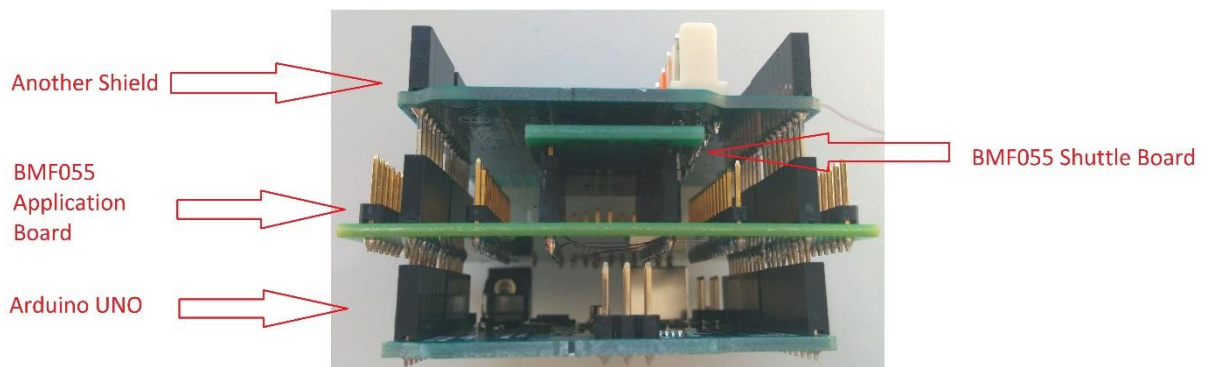
Figure 4 - Connection to Arduino UNO and an Arduino shield
