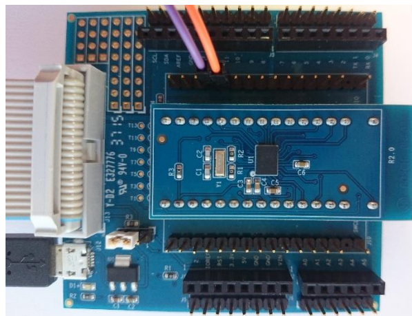
Figure 6 - Necessary connections to run reference examples
