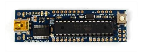
Next, you can attach header pins to make the USB Boarduino fit nicely into a breadboard. If you want to solder wires to the pins instead (free-wiring) you should skip this step.
