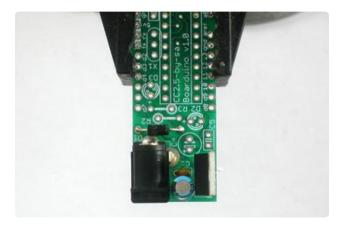
Next is the 5V regulator. This takes the power from the DC jack which may be something like a 9V battery, and brings it down to 5V, which is suitable for the microcontroller chip. This part must be placed as shown, with the metal heat sink tab on the right.
