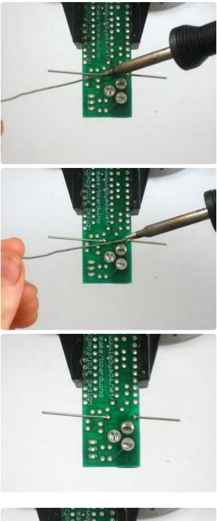
Turn the PCB over and solder both legs so that you get a nice shiny solder joint.
