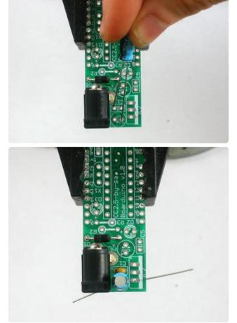
Next, its time to place the 25V electrolytic capacitor C3. Electrolytic capacitors are polarized which means they only work well in one direction. Put it in backwards and they can explode! You can tell how to place it because the silkscreened image has a plus near one hole and the capacitor has one long lead. That lead is the positive lead. In this image, its the one on the right.
