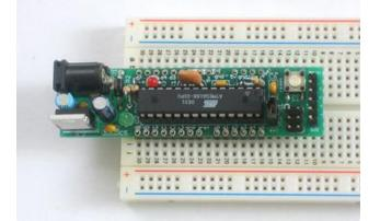
Place the Boarduino on top, so that the header matches up with the solder holes in the PCB.
