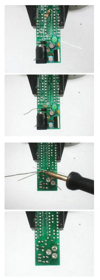
The 1K resistor R2 goes in, its the LED's matching resistor. Bend it over as shown to place it.
