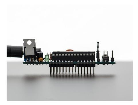
The Boarduino is an Arduino clone: when programmed with the Arduino bootloader, it can talk to the Arduino software and run sketches just like the original.
