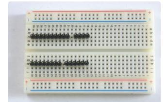
Cut 4 more pieces of header, a 10-pin, 8pin, 6-pin and 4-pin. Insert them into a solderless breadboard as shown so that the long legs are in the solderless breadboard sockets.
