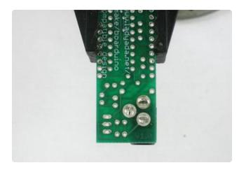
Make sure all three pads are soldered, with plenty of solder, the holes should be filled up. This gives the jack mechanical strength.
