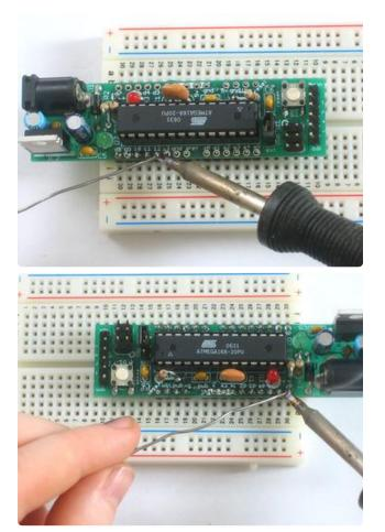
Solder all of the pins of the header, making sure that the board is sitting flat against the header.
