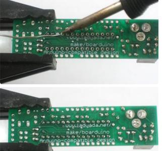
Solder in the socket by tacking two opposite corners and then soldering the rest of the pins. Press the socket into the board to make sure its flat up against it.
