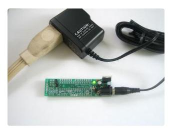
Take the board out of the vise and plug in a power source such as a 9V DC positivetip wall adapter or a 9V battery with a 2.1mm barrel jack. You should see the green LED light up.
