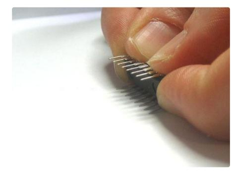
Once the pins are straight, insert the chip by matching the U notch in the chip with the U notch in the socket.
