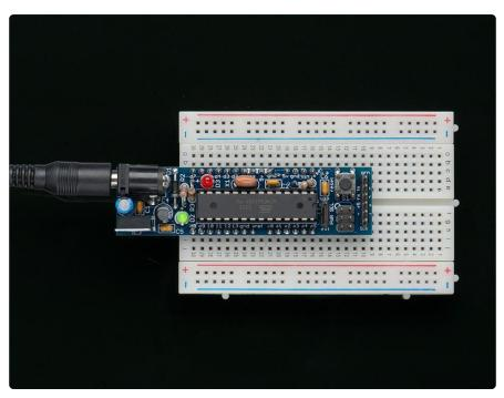
If you've ever struggled to use a solderless breadboard with an Arduino, you understand how frustrating it can be! I designed this Arduino clone to solve this problem in an inexpensive DIY fashion.
