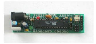
If you'd like to take advantage of the autoreset capabilities added to the Arduino software, install ceramic capacitor C6.
