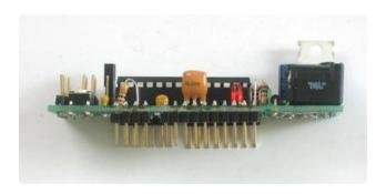
Carefully remove the boarduino by slowly rocking it back and forth to release it from the solderless breadboard.
