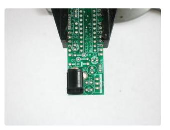
Place the 2.1mm DC jack as shown, it should fit in snugly. Make sure the part is on the top of the board, so that you can see the silkscreened images.
