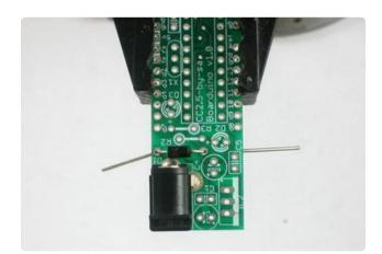
Next, place the 1N4001 diode D1 . Diodes are directional, they only let current flow in one direction. This diode is used to protect the Boarduino from damage. Make sure the white stripe on the diode matches the white stripe in the silkscreened image below. In this picture, the stripe is on the right.
