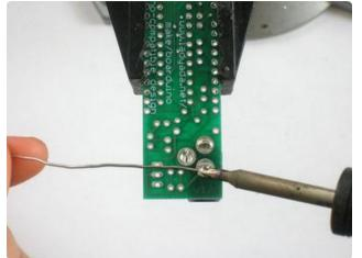
Use the soldering iron to heat up each of the 3 connections and poke the solder in so that it melts into the holes.
