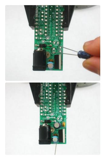
Now you should soder in the 6.3V electrolytic capacitor C4 as shown. Remember its polarized so you must place the longer lead in the positive-marked hole.
