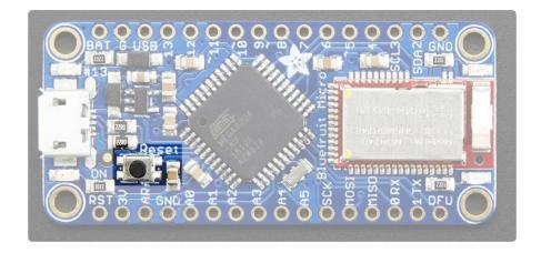
To the right is a small tactile switch. This is the reset button for the ATmega32u4. You can use this to reset the microcontroller and/or push it into bootloader mode if the bootloader gets 'stuck' during programming
