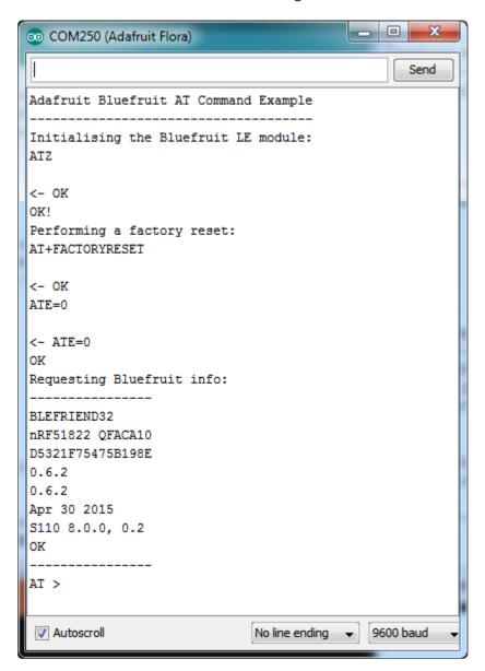
To send an AT command to the Bluefruit LE module, enter the command in the textbox at the top of the Serial Monitor and click the Send button:
