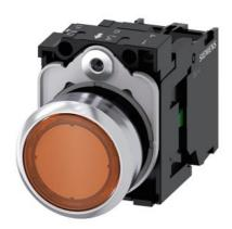
Illuminated pushbutton, 22 mm, round, metal, shiny, amber, pushbutton, flat, momentary contact type, with holder, 1NO, LED module with integrated LED 230 V AC, screw terminal, with laser labeling, upper case and lower case, always upper case at beginning of line
