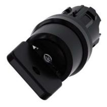
Key-operated switch O.M.R, 22 mm, round, plastic, lock number 73034, black, with 2 keys, 2 switch positions O-I, latching, actuating angle  $90^\circ, 10:30h/13:30h$ , key removal O+I, with laser labeling, upper case and lower case, always upper case at the beginning of the word
