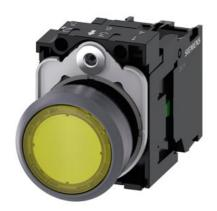
Illuminated pushbutton, 22 mm, round, plastic with metal front ring, yellow, pushbutton, flat, momentary contact type, with holder, 1NO, LED module with integrated LED 230 V AC, screw terminal, with laser labeling, lower case
