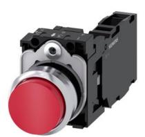
Pushbutton, 22 mm, round, metal, shiny, red, pushbutton, raised, momentary contact type, with holder, 1 NO+1 NC, screw terminal, with laser labeling, symbol number according to, ISO 7000 or IEC 60417
