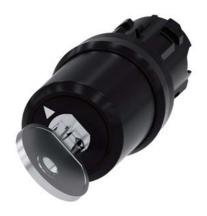
Key-operated switch BKS, 22 mm, round, plastic, Lock No. E2 (VW), without key, 2 switch positions O-I, latching, actuating angle 90°, 10:30h/13:30h, key removal O+I, with laser labeling, upper case and lower case, always upper case at beginning of line
