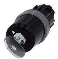
Key-operated switch BKS, 22 mm, round, plastic with metal front ring, Lock No. E7 (VW), without key, 2 switch positions O-I, latching, actuating angle 90°, 10:30h/13:30h, key removal O, with laser labeling, upper case and lower case, always upper case at the beginning of the word
